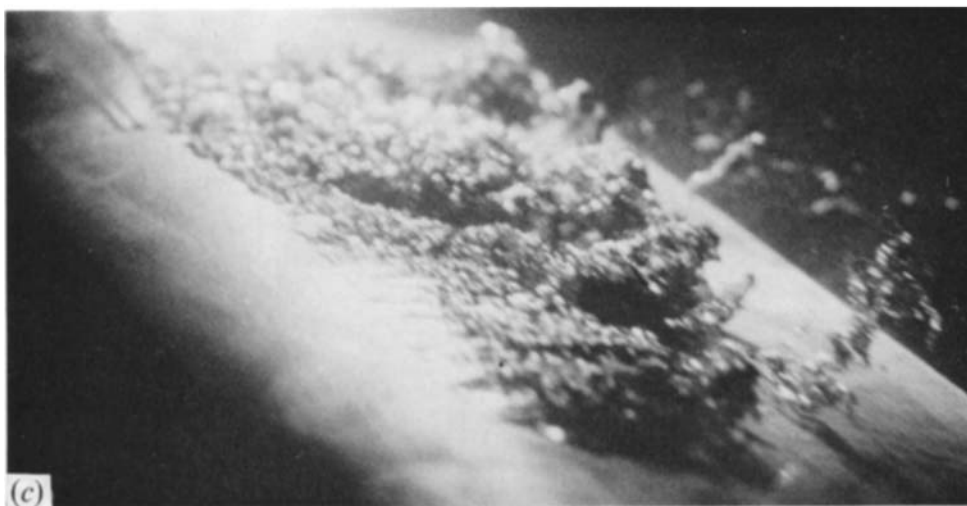
FIGURE 4. Representative photographs of cavitation without boundary-layer tripping. (a), (b) \sigma = 1.15 with U_\infty = 16 ft/s. (c) \sigma = 0.74 with U_\infty = 20 ft/s.
